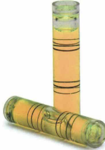
Barrel vials are curved only on the inside. Molded-barrel vials of acrylic plastic are cheap to make, and they can be read in any position. Manufacturers can substitute a single-barrel vial for two curved vials.
